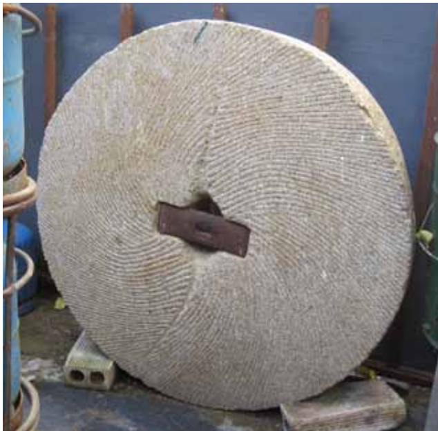
Example of a granite millstone in a local Gerena watermill. The stone, dressed with arc-shaped furrows, is presumably from a local quarry (photograph by Lucas Acuña Carabantes).
