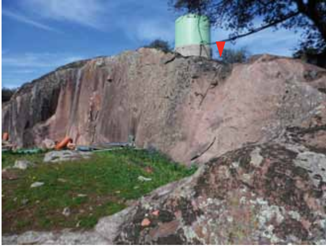
View of extraction sector 1 of the quarry. This quarry face bears scars of long vertical drilling holes indicating very recent work probably with black powder (photograph by Silverio Gutiérrez).
