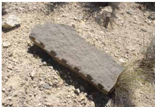
Large blocks were reduced by wedging before being hewn into cobblestones.
