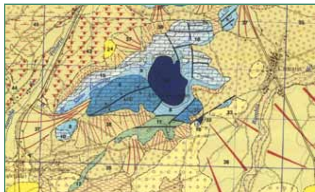
Extract from geological map 868 (IGME). The dark unit is "Jumillita" volcanic rock and is the presumed location of the quarry. More recent geological research defines the rock as a lamproite, a type known to have been exploited since Roman times for querns and millstones.
